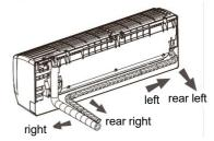
When select leading out the pipe from left or right, please cut off the corresponding hole on the bottomcase.
